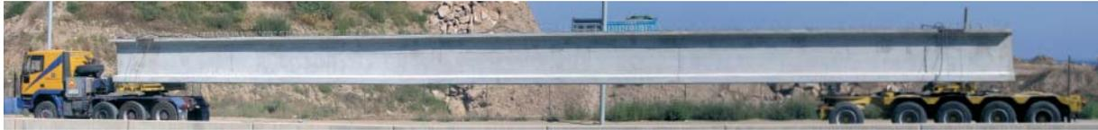
Fig. 25: Transport of a large I-beam by road
